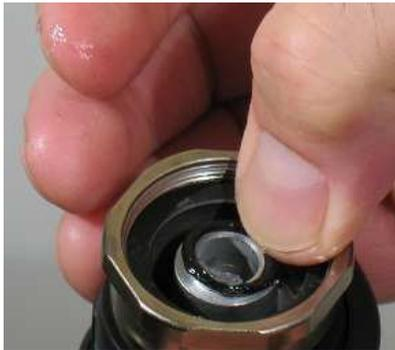
7. Apply a small amount of Loctite Primer #7649 to the threads of the **01546/50776** Housing.
