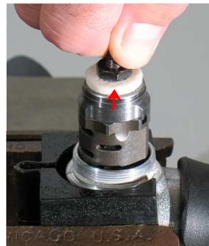
4. Remove the motor from the housing.
