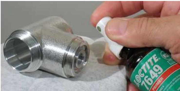
8. Apply a small amount of Loctite #567 to the housing.
