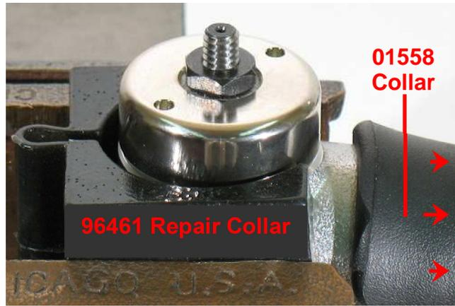
2. Pull the **01558** Collar back onto the throttle body housing. Use the **96460** Wrench to loosen the throttle body from the 7° housing. **Left Hand Thread** Turn clockwise.
