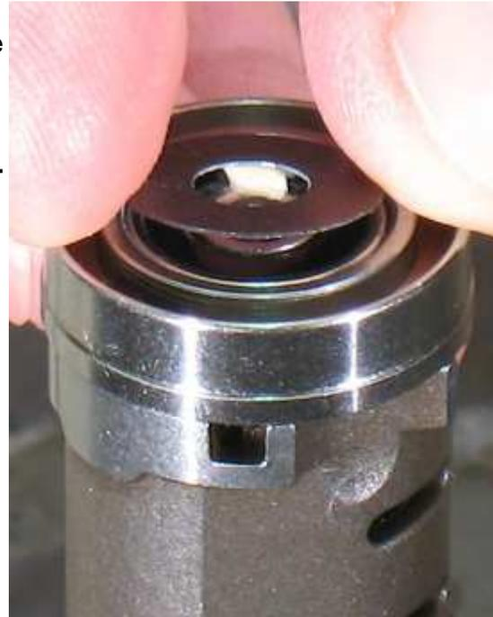
13. Apply a small amount of Loctite Primer # 7649 to the threads of the **01546/50776** Housing. Apply a small amount of Loctite #567 to the housing.
