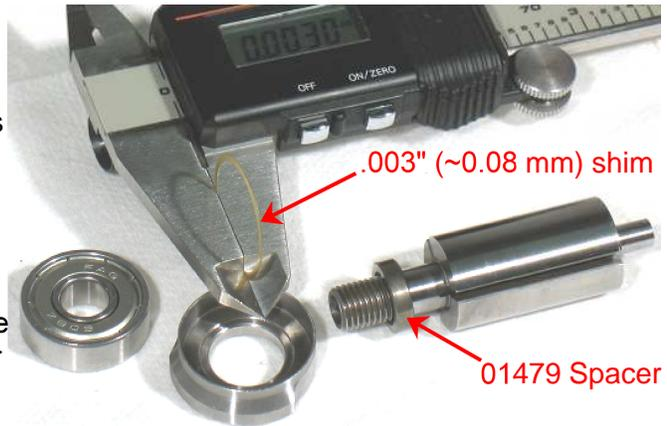
4. Fasten the rotor in the vise with aluminum or bronze jaws so that the spindle is pointing up. Use a 12 mm socket and torque wrench to install the **50133** Adapter or **01435** Collet Body. Turn clockwise. (T 17 N•m/~150 in. lbs.)
