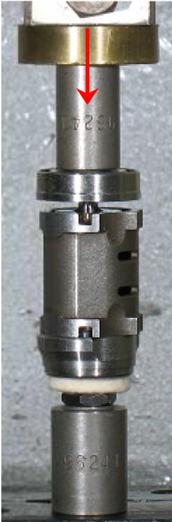
10. Use the **RAISED CENTER** of the **96242** Bearing Press Tool and the arbor press to install the **02696** Bearing onto the rotor, and into the **02673** Rear Bearing Plate.
