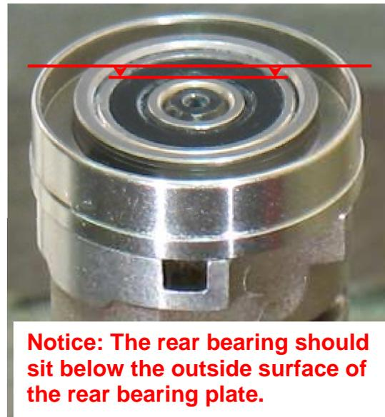
11. If the model contains a **02679** Shield, place a small amount of clean grease on the seal of the **02696** Bearing and stick the shield against the bearing.
