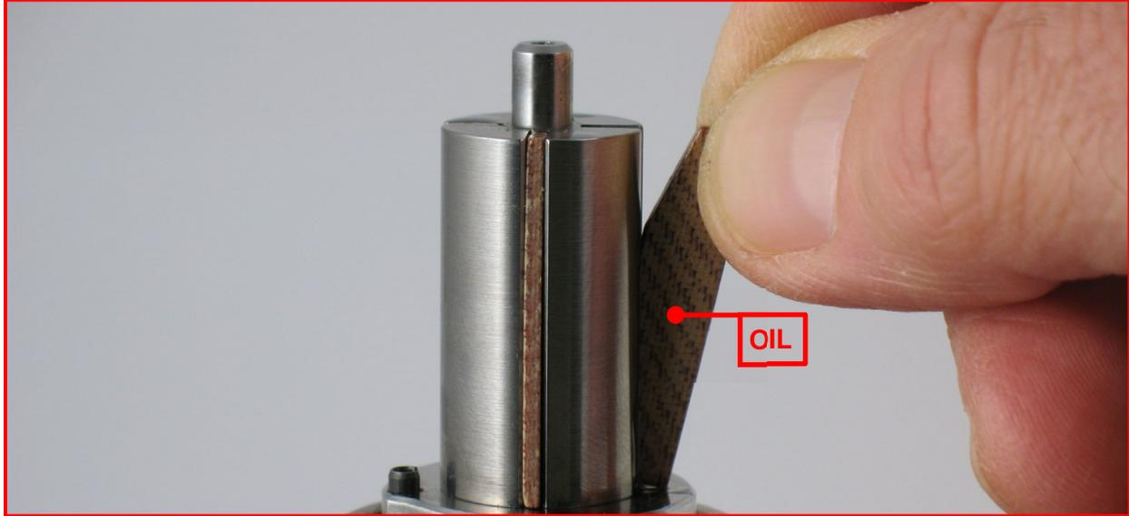
5. Lubricate the **01480** Vanes with the **95842** Dynabrade Air Lube 10W/NR or equivalent.
