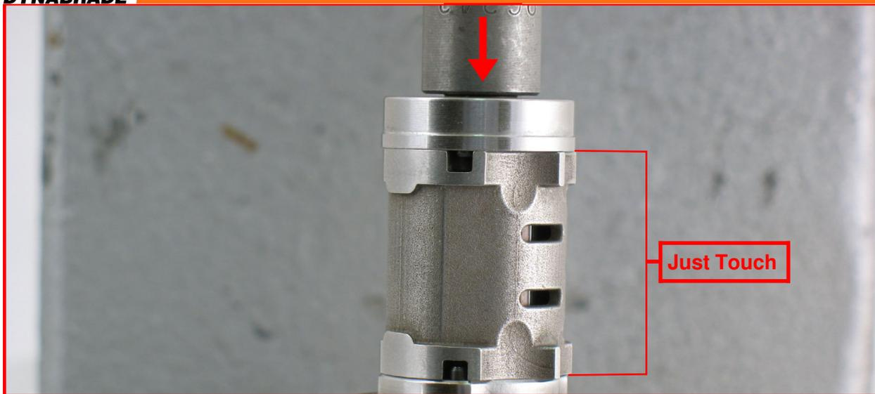
8. Use the **RAISED INSIDE DIAMETER** of the **96242** Bearing Press Tool and the arbor press to install the rear bearing and plate onto the rotor. **Notice:** Carefully press the bearing and plate down until it just touches the cylinder. This will establish a close fit between the bearing plates and the cylinder.
