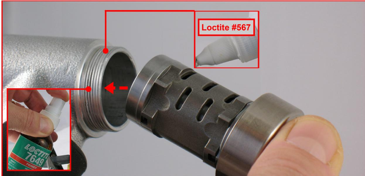
10. Carefully install the motor assembly into the **01546** Housing.
