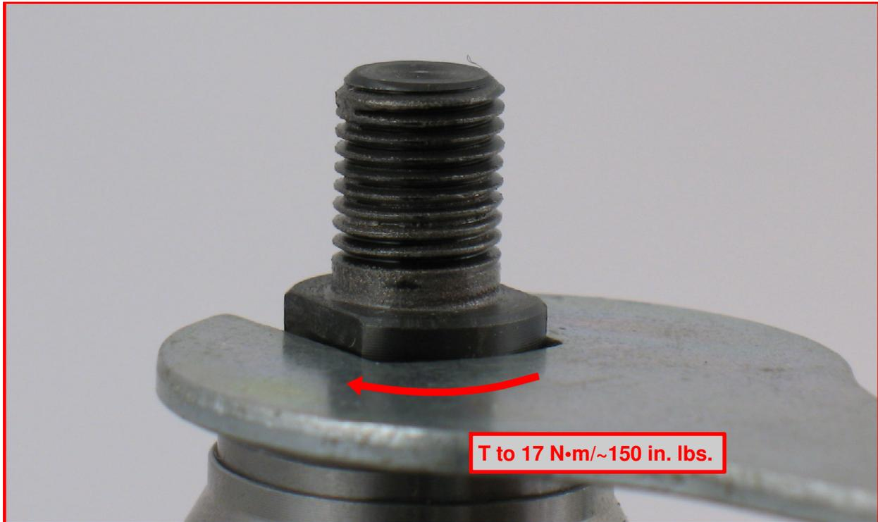
4. Once the correct clearance is achieved, fasten rotor in vise and tighten the **04117** Adapter.
