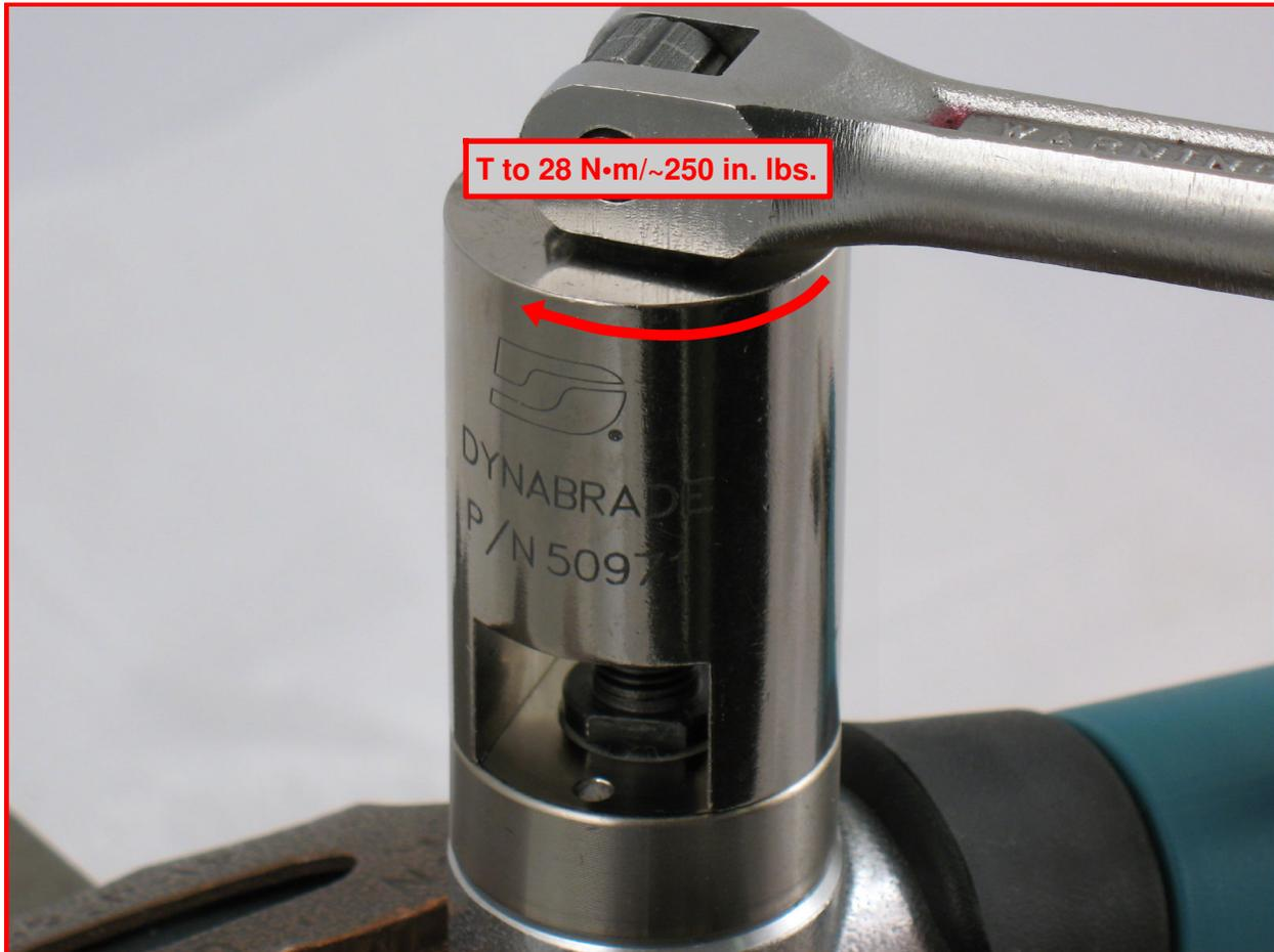
11. Carefully fasten the **01546** Housing in the vise with aluminum or bronze jaws so that the **04117** Adapter is pointing up. **Notice: Over tightening vise will damage housing.** Repair Collar **96461** (designed to protect the **01546** Housing) is available upon order.
