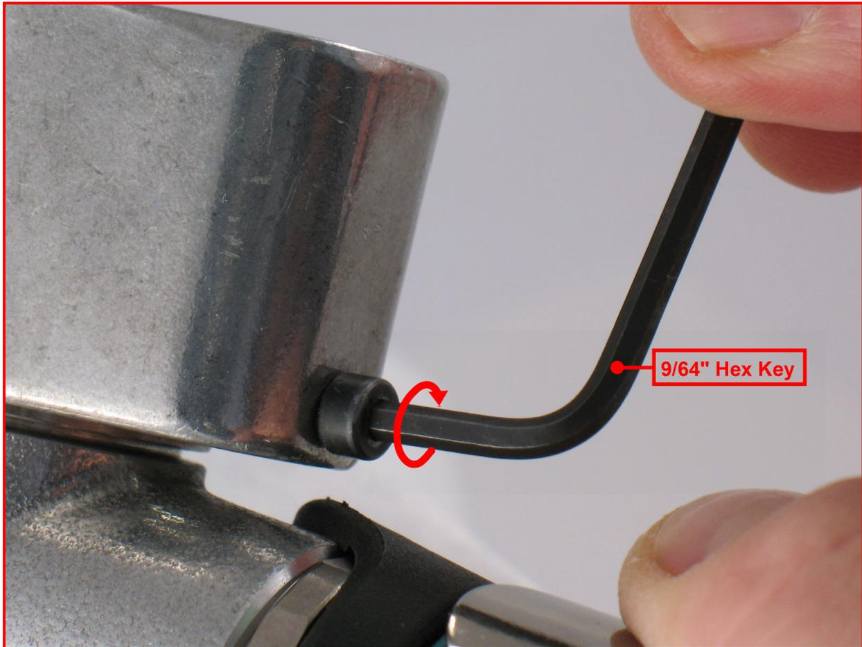
12. Install air motor into the belt housing assembly.
