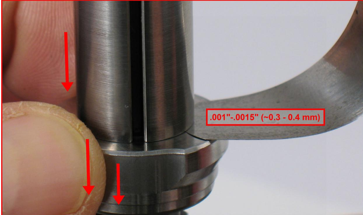
3. Use a .001" (~0.3 mm) thick feeler gauge to check clearance between the front bearing plate and the front of the rotor.
