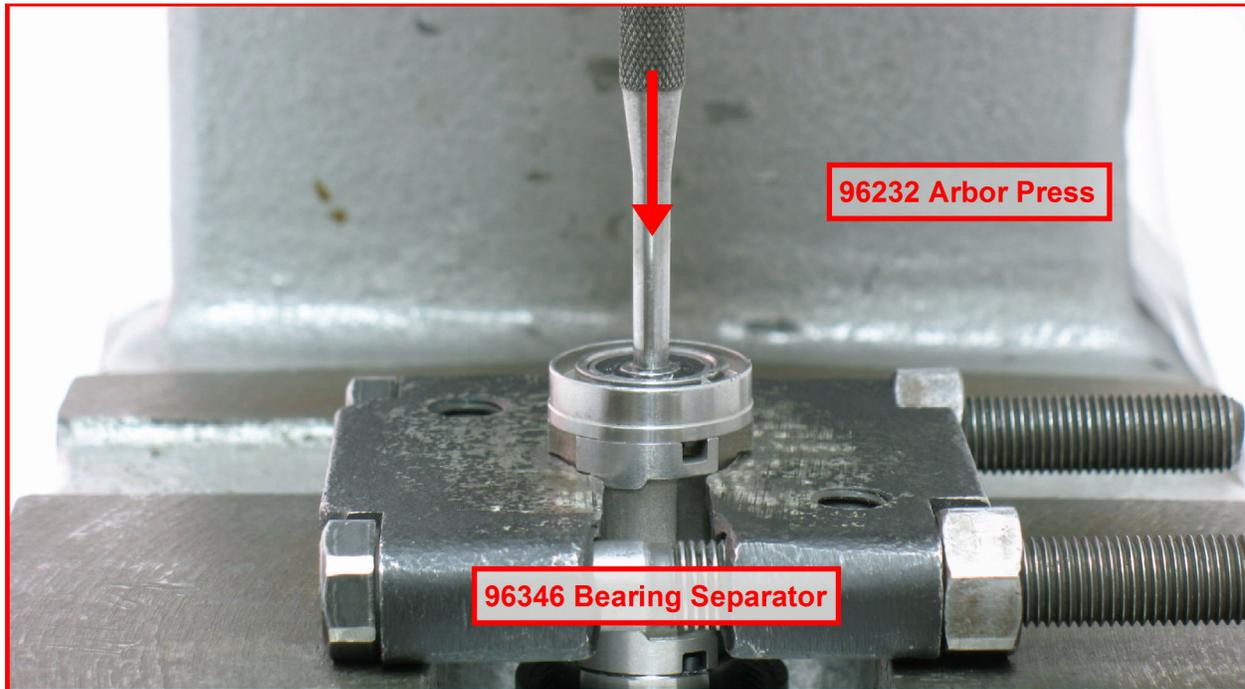
5. Fasten the **96346** Bearing Separator (2") around the **01476** Cylinder.
