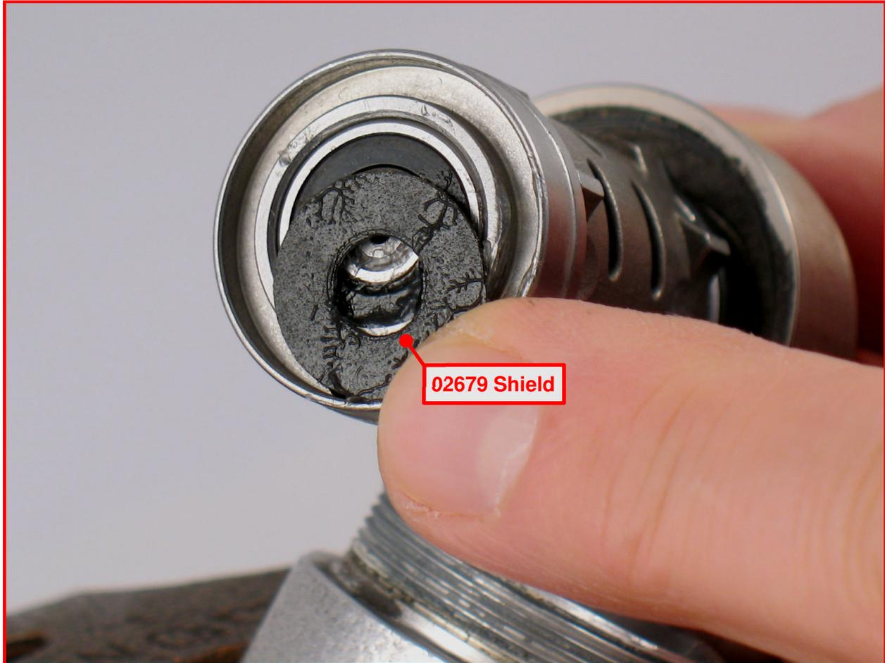
4. Loosen the vise and carefully pull the motor out of the **01546** Housing.
