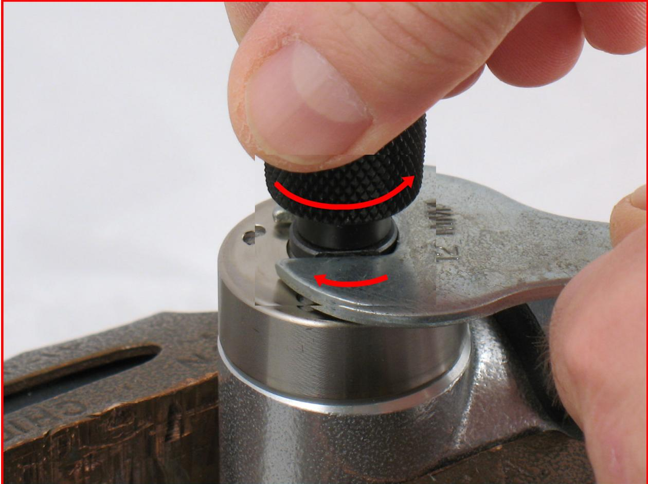
2. Carefully fasten the **01546** Housing in a vise with aluminum or bronze jaws so that the drive wheel is pointing up. **Notice: Over tightening vise will damage housing.** Repair Collar **96461** (designed to protect the **01546** Housing) is available upon order.
