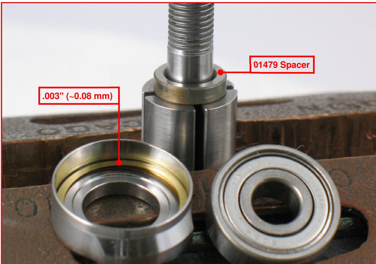
1. Fasten the rotor in a vise with aluminum or bronze jaws so that the rotor spindle is pointing up.
