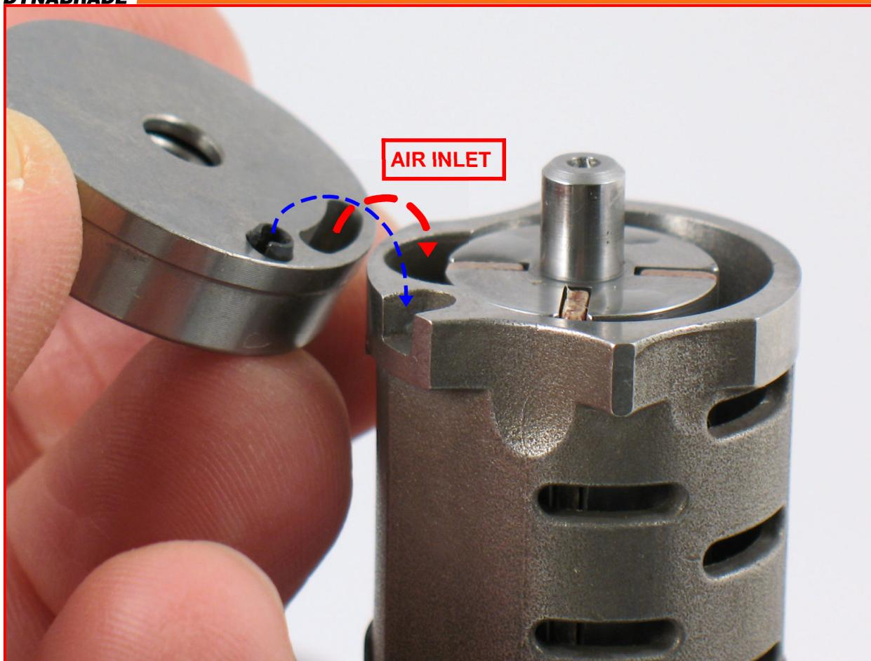
7. Install the **01476** Cylinder so that the air inlet opening in the **02673** Rear Bearing Plate will line up with the air inlet opening of the cylinder.
