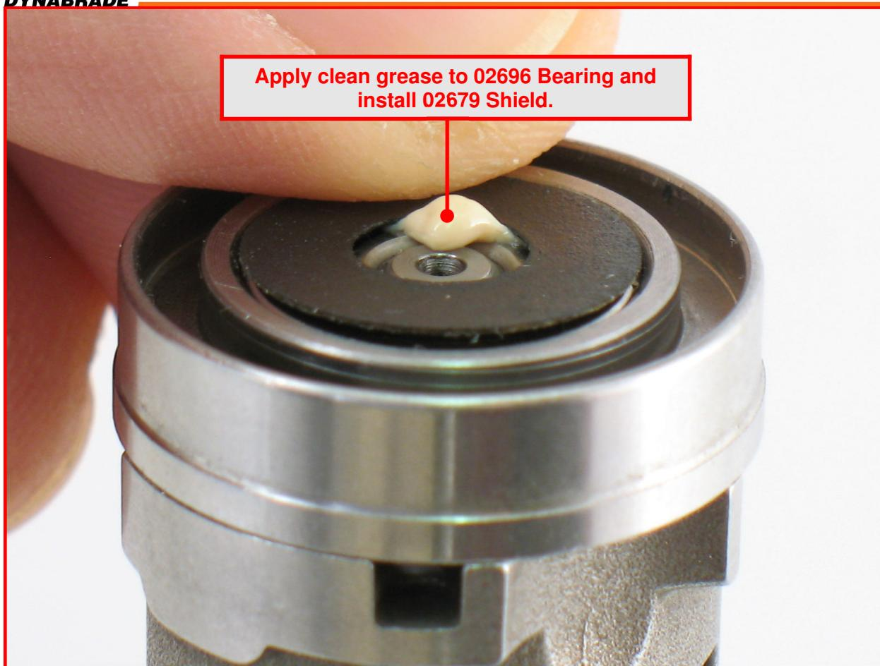
9. Apply a small amount of clean grease to the seal of the **02696** Bearing. **Notice:** The grease is used to hold the shield against the seal of the bearing.
