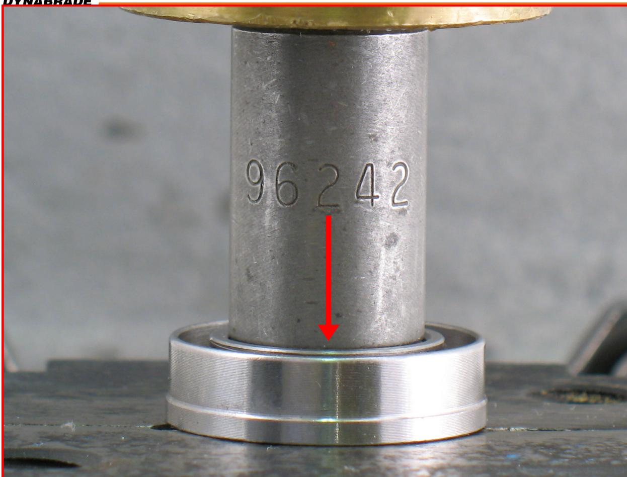
6. Use the **RAISED OUTSIDE DIAMETER** of the **96242** Bearing Press Tool and the **94232** Arbor Press (#2) to install the **02696** Bearing into the **02673** Rear Bearing Plate.
