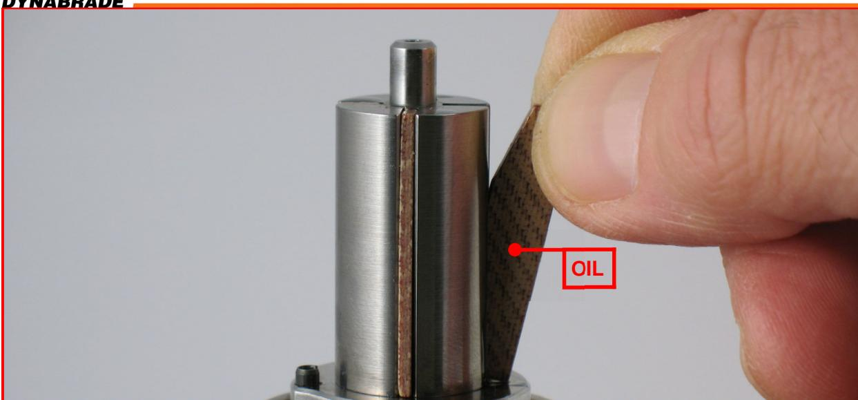
5. Lubricate the **01480** Vanes with the **95842** Dynabrade Air Lube 10W/NR or equivalent.
