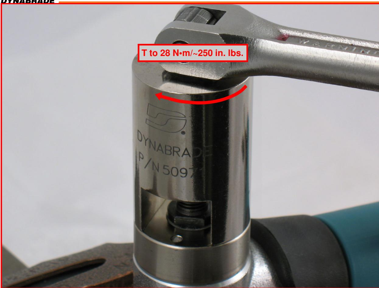
11. Carefully fasten the **01546** Housing in the vise with aluminum or bronze jaws so that the **04117** Adapter is pointing up. **Notice: Over tightening vise will damage housing.** Repair Collar **96461** (designed to protect the **01546** Housing) is available upon order.
