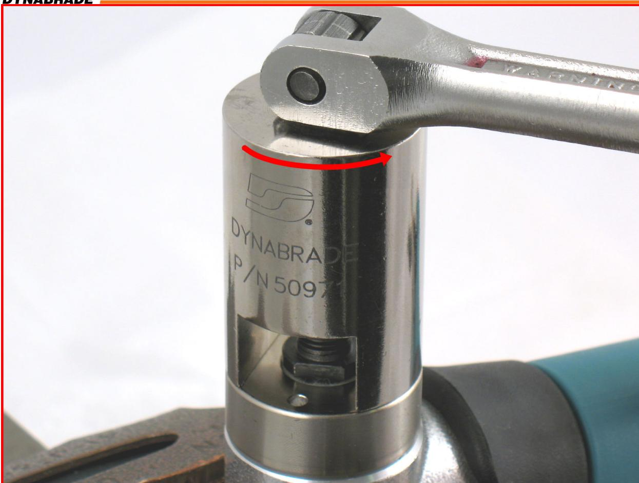
3. Use the **50971** Lock Ring Tool or an adjustable 3 mm pin spanner wrench to remove the **04116** Exhaust Cover. Turn counterclockwise.
