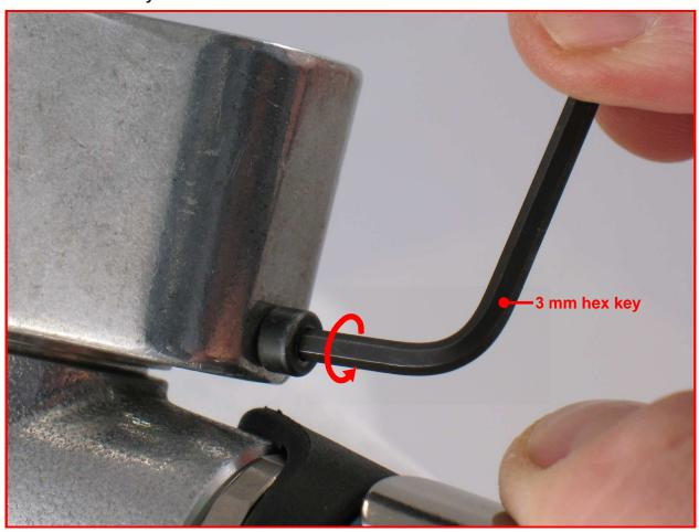
1. Use a 3 mm hex key to loosen the **01788** Motor Lock Screw. Remove the **15060** Housing Assembly from the air motor.
