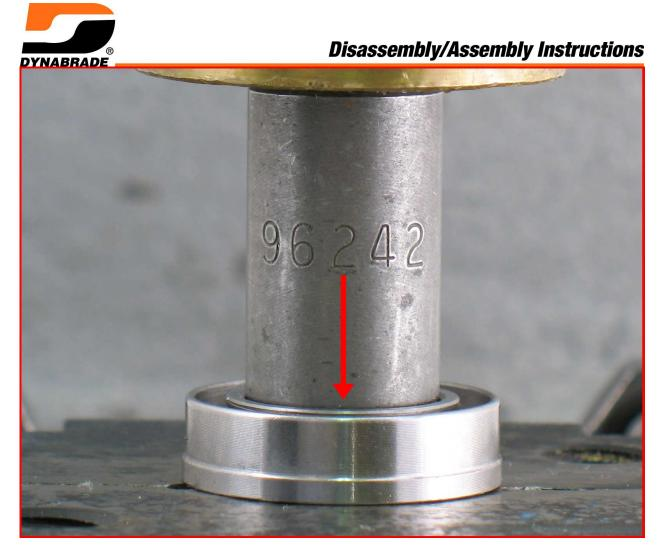
**6.** Use the **RAISED OUTSIDE DIAMETER** of the **96242** Bearing Press Tool and the **94232** Arbor Press (#2) to install the **02696** Bearing into the **02673** Rear Bearing Plate.
