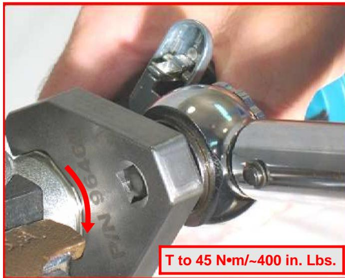
6. Install the throttle body onto the 7° housing.
