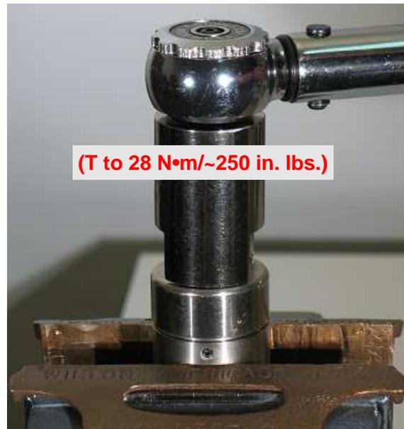
**Planetary Gear Assembly Complete.**
