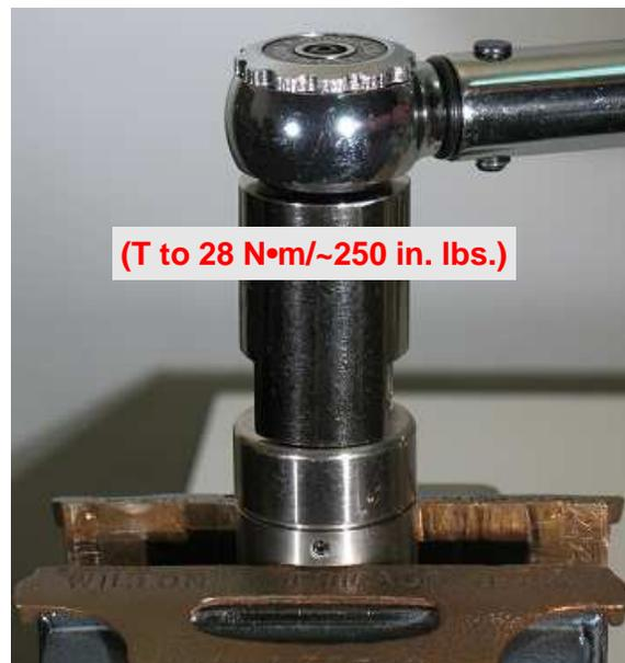
**Planetary Gear Assembly Complete.**
