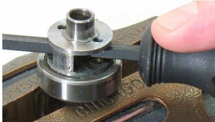
9. Use the arbor press, and a 5/16" flat-end drive punch as a press tool to push the planetary carrier out of the remaining **54520** Bearing.
