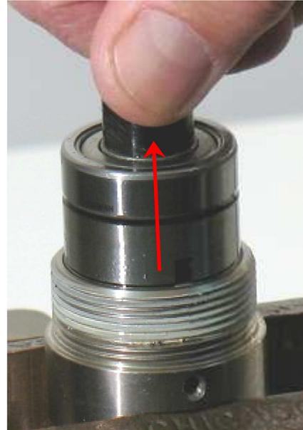
7. Remove the ring gear, shafts, and planet gears.
