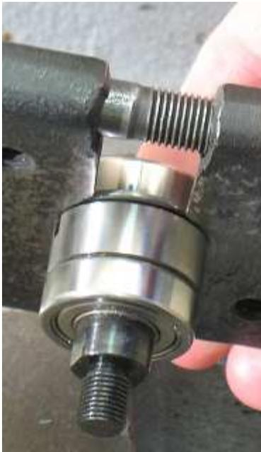
6. Use a 5/16" flat-end drive punch as a press tool to push the planetary carrier out of the **54520** Bearing.
