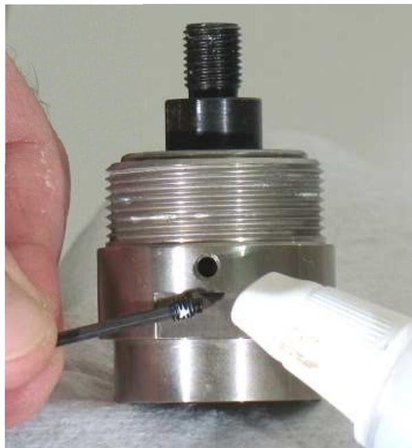
6. Apply Loctite #7649 Primer, and a small amount of Loctite #567 (or equivalent) to the threads of the adapter or gear case.
