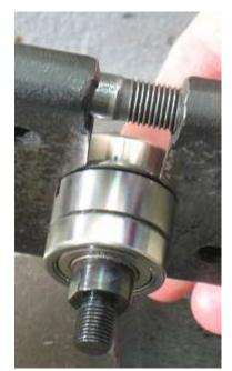
drive punch as a press tool to push the planetary carrier out of the **54520** Bearing.
