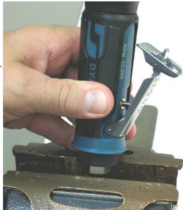
**Notice:** If the **01578** or **94523** Inlet Adapter loosens before the rear exhaust cover or planetary housing, remove the inlet adapter, muffler and valve parts. Fasten the **96399** Hex Key (12 mm) in the vise with the notched end pointing up.
