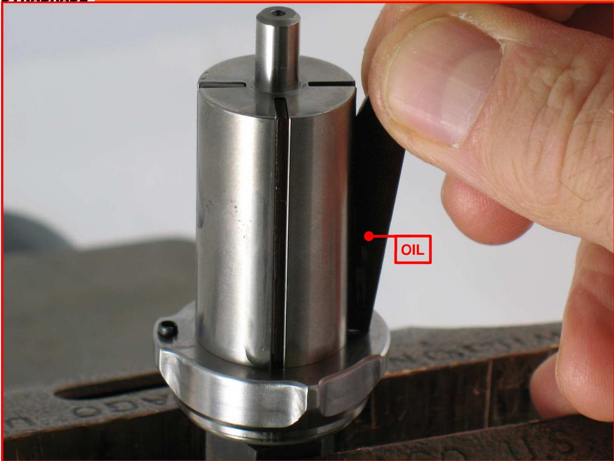
4. Apply the **95842** Dynabrade Air Lube, 10W/NR or equivalent to the **01011** Vanes and install them into the rotor.
