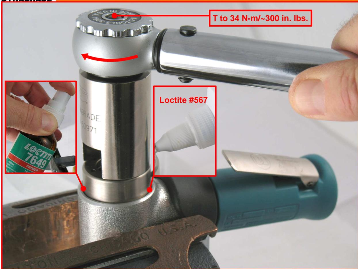
9. Carefully fasten the **01447** Housing in a vise with aluminum or bronze jaws so that the rotor spindle is pointing up. **Notice: Over tightening vise will damage housing.**
