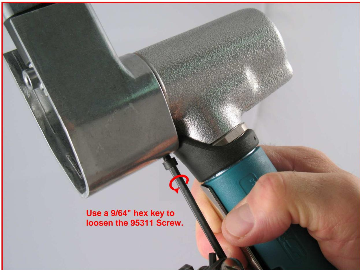
1. Use a 9/64" hex key to loosen the 95311 Screw. Remove the motor from the belt housing.
