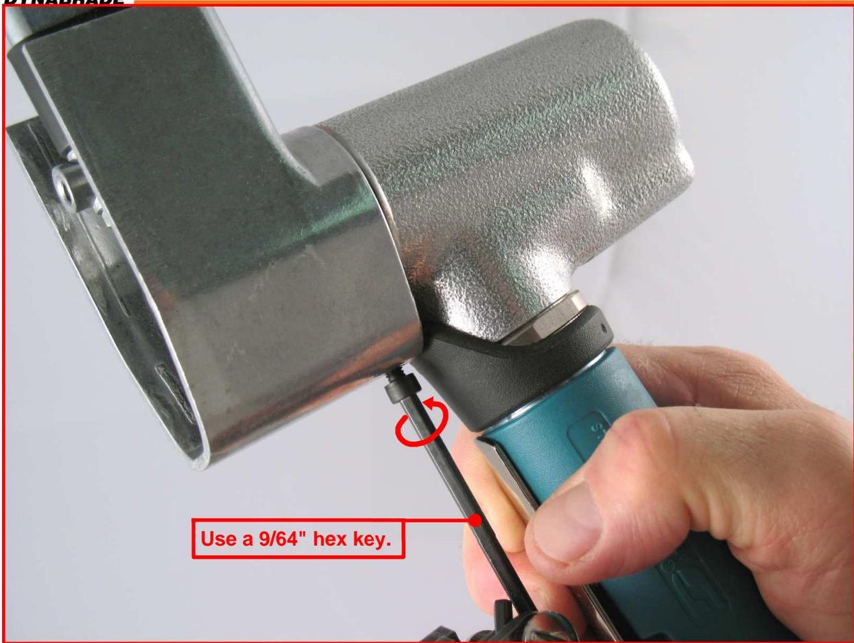
11. Install the air motor into the housing.
