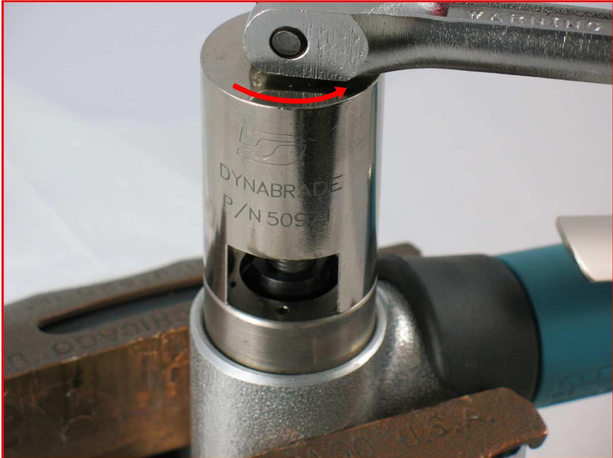
3. Use the **50971** Lock Ring Wrench to remove the motor lock ring. Turn counterclockwise.
