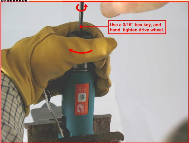
**10.** Insert a 3/16" hex key through the **01111** Drive Wheel and into the end of the **01120** Rotor to hold it stationary.
