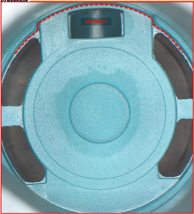
8. Important: Line-up the air inlet of the rear bearing plate with the air inlet in the housing.
