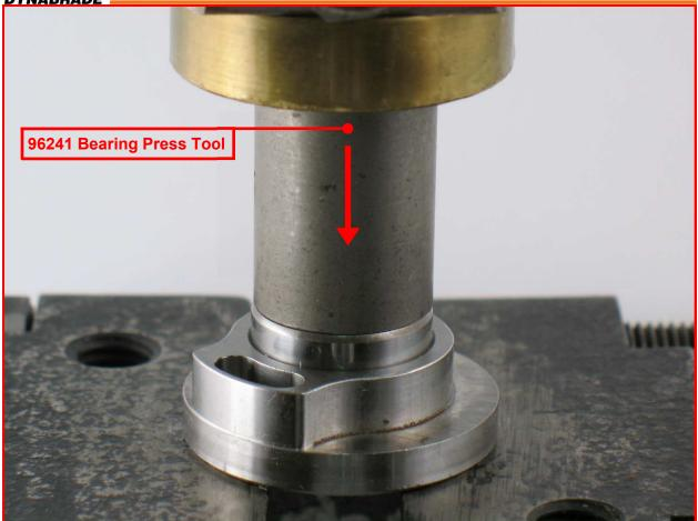
5. Use the **RAISED OUTSIDE DIAMETER** of the **96241** Bearing Press Tool and the arbor press to install the **01015** Bearing. **Notice:** Press the bearing all the way into the plate.
