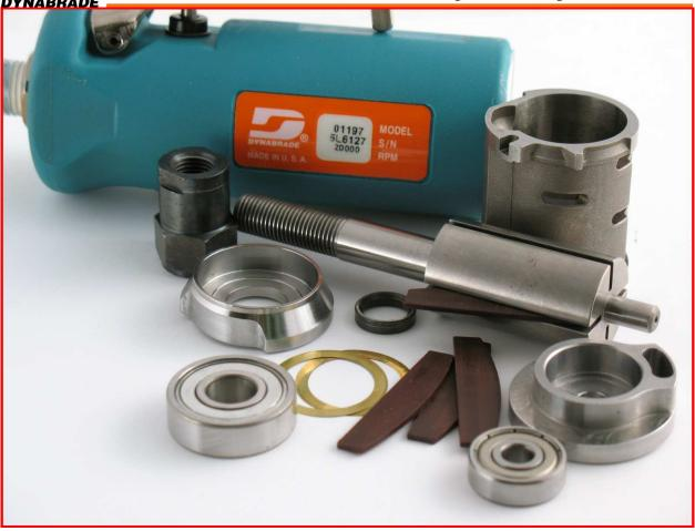
Motor Disassembly Completed.
