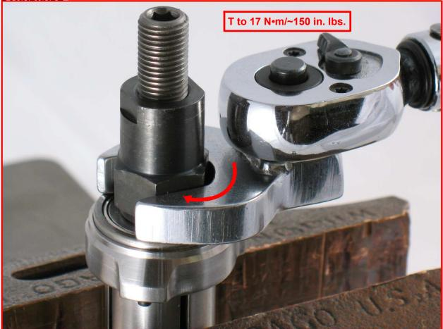
Use a 17 mm socket or crowfoot, and a torque wrench to tighten the 04081 Rotor Nut. (T to 17 N•m/~150 in. lbs.)
