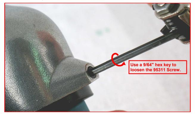
1. Use a 9/64" hex key to loosen the **95311** Screw. Remove the **01197** Air Motor along with the **11424** Wave Spring and the **11419** Cover.
