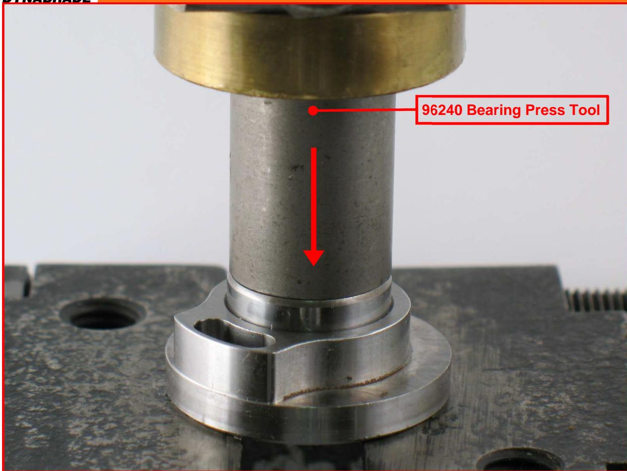
5. Use the **RAISED OUTSIDE DIAMETER** of the **96240** Bearing Press Tool and the arbor press to install the **02649** Bearing. **Notice:** Press the bearing all the way into the plate.
