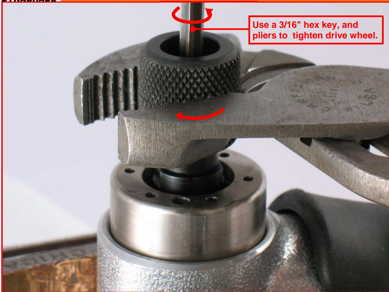
10. Insert a 3/16" hex key through the drive wheel and into the end of the **55025** Rotor to hold it stationary.
