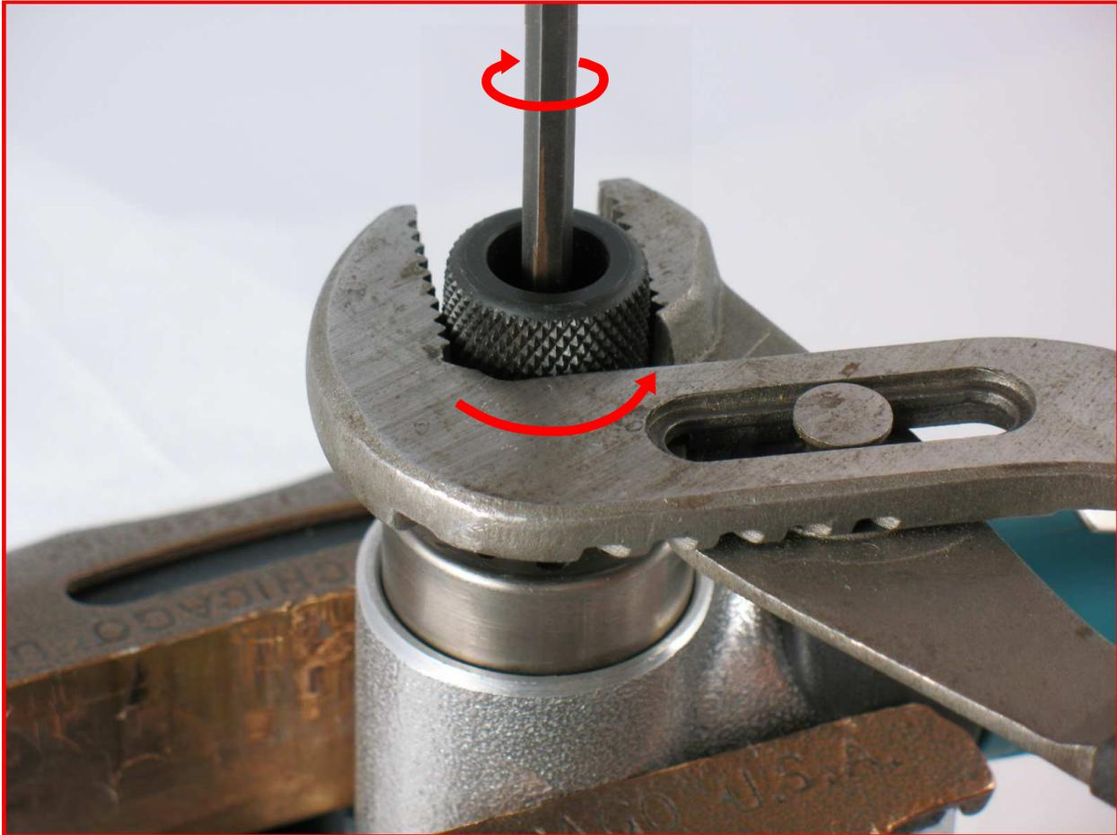
2. Carefully hold the **01739** Housing in a vise with aluminum or bronze jaws so that the drive wheel is pointing up. **Notice: Over tightening vise will damage housing.**
