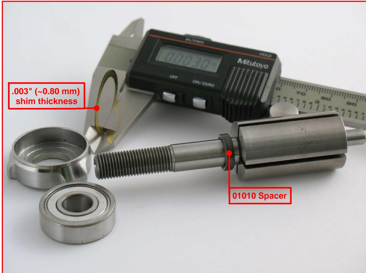
1. Install the **01010** Spacer onto the rotor.
