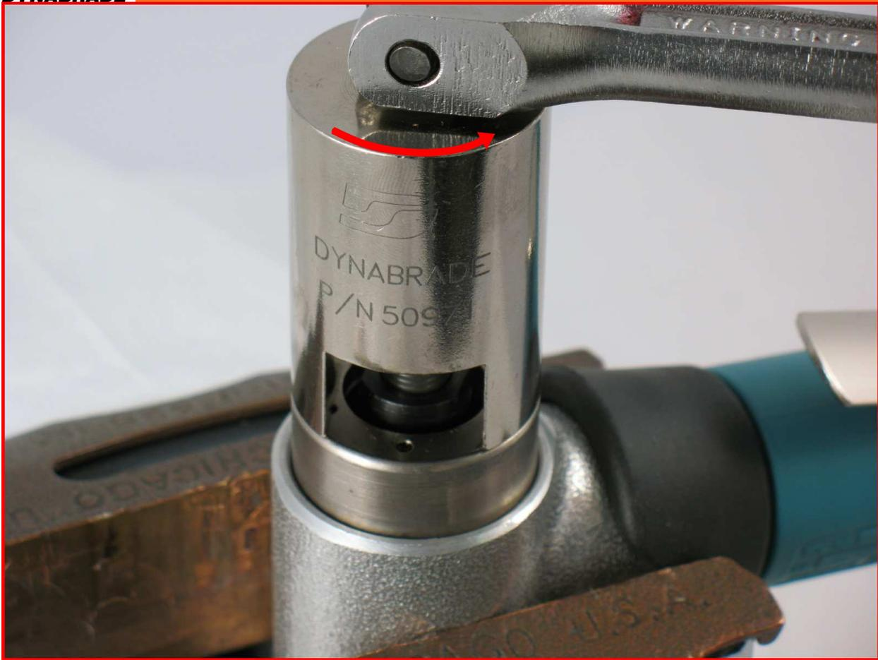
3. Use the **50971** Pin Wrench to remove the **15315** Exhaust Cover. Turn counterclockwise.
