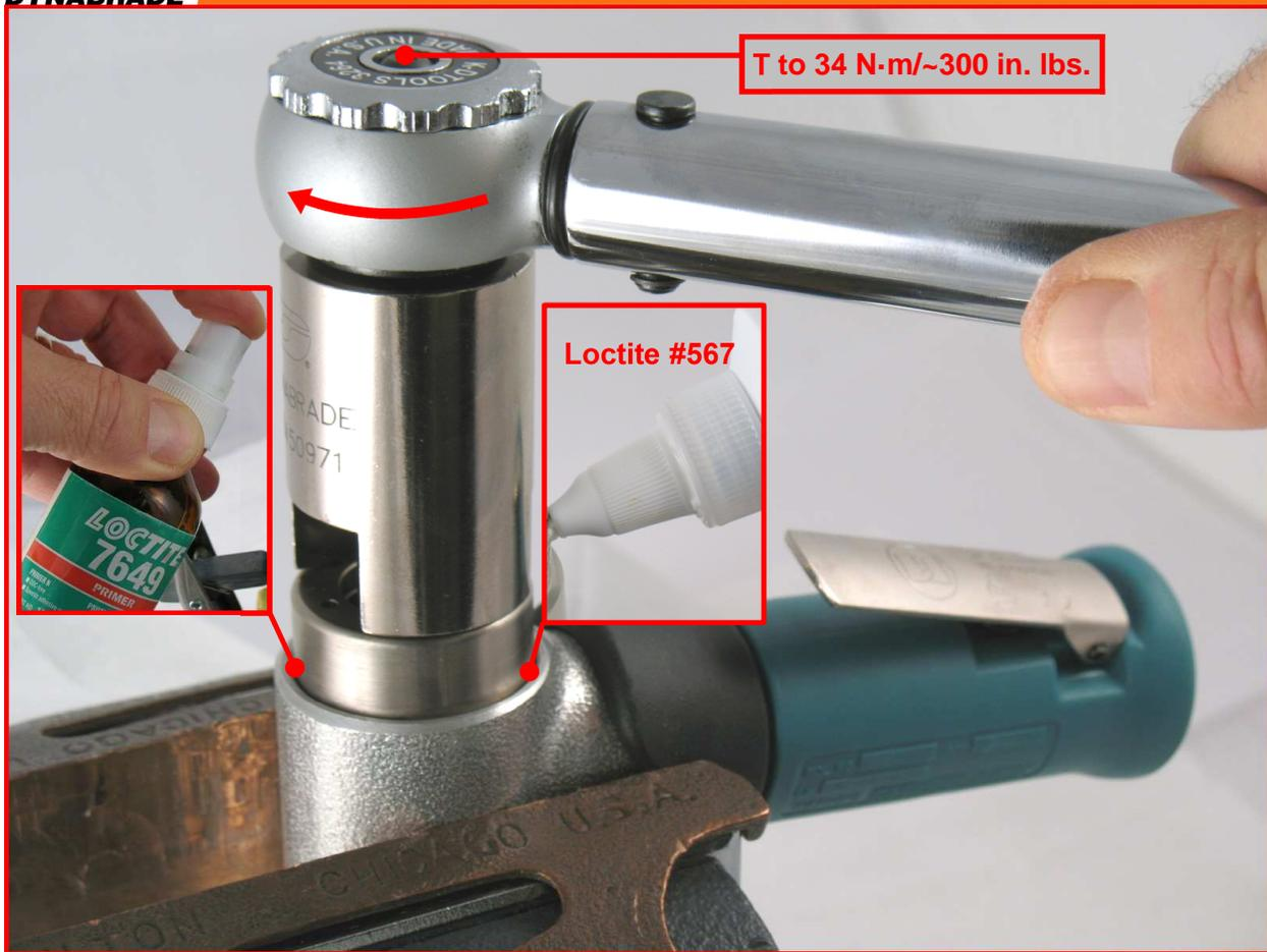
9. Carefully fasten the **01739** Housing in the vise with aluminum or bronze jaws so that the rotor spindle is pointing up. **Notice: Over tightening vise will damage housing.**
