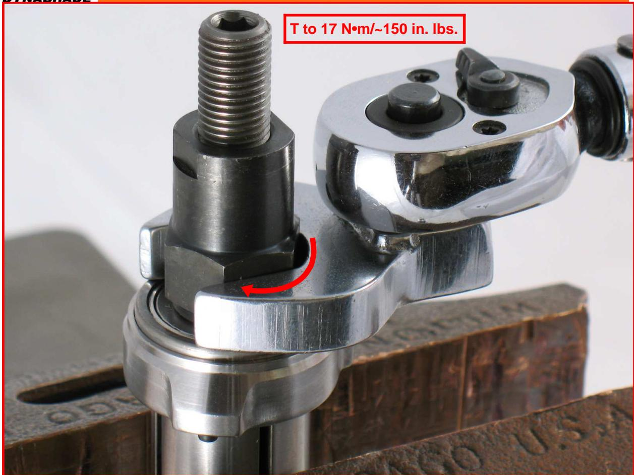
3. Use a 19 mm crowfoot and a torque wrench to tighten the **01708 Rotor Nut**.
