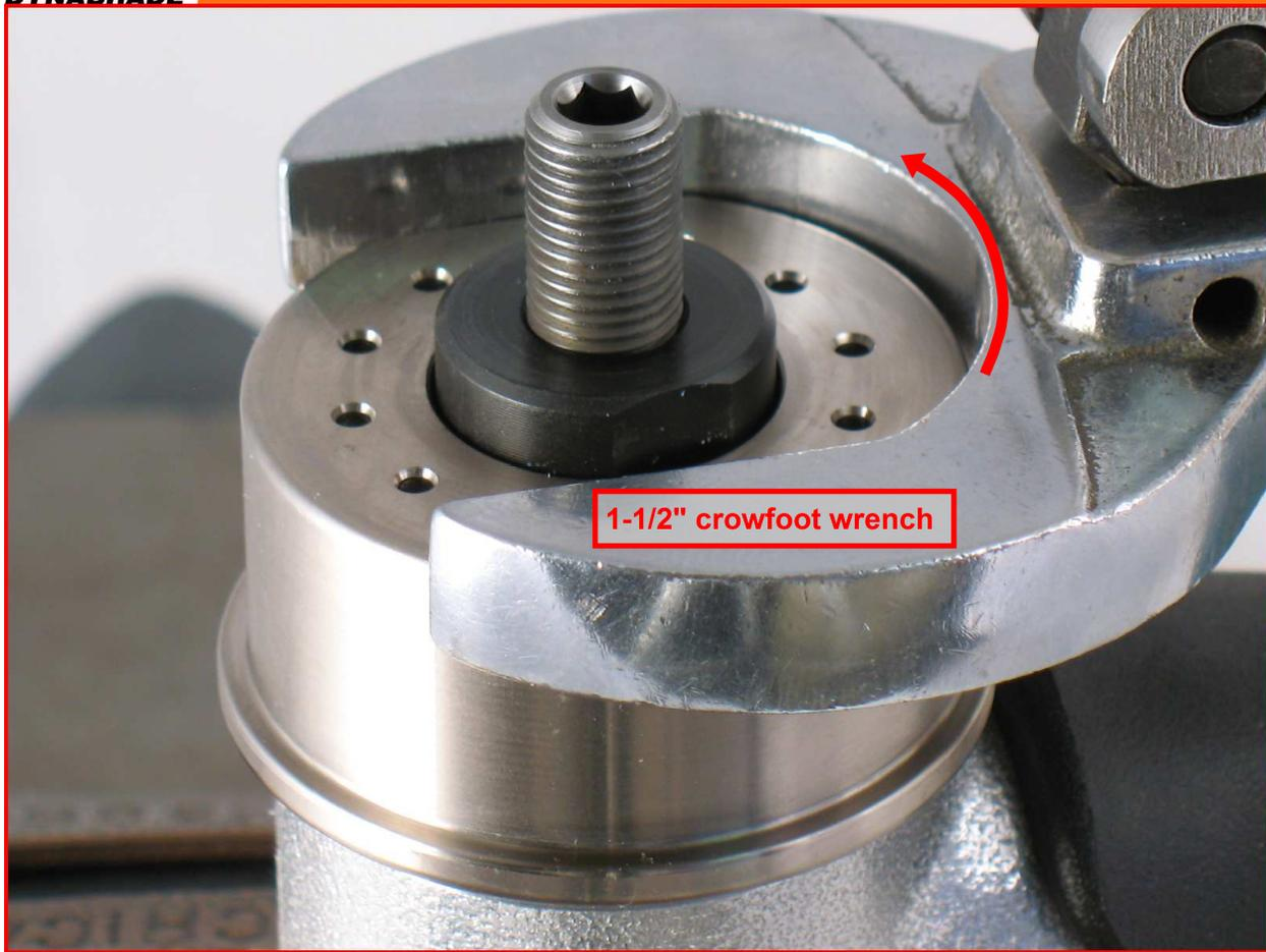
3. Carefully fasten the **01739** Housing in a vise with aluminum or bronze jaws so that the spindle is pointing up.
