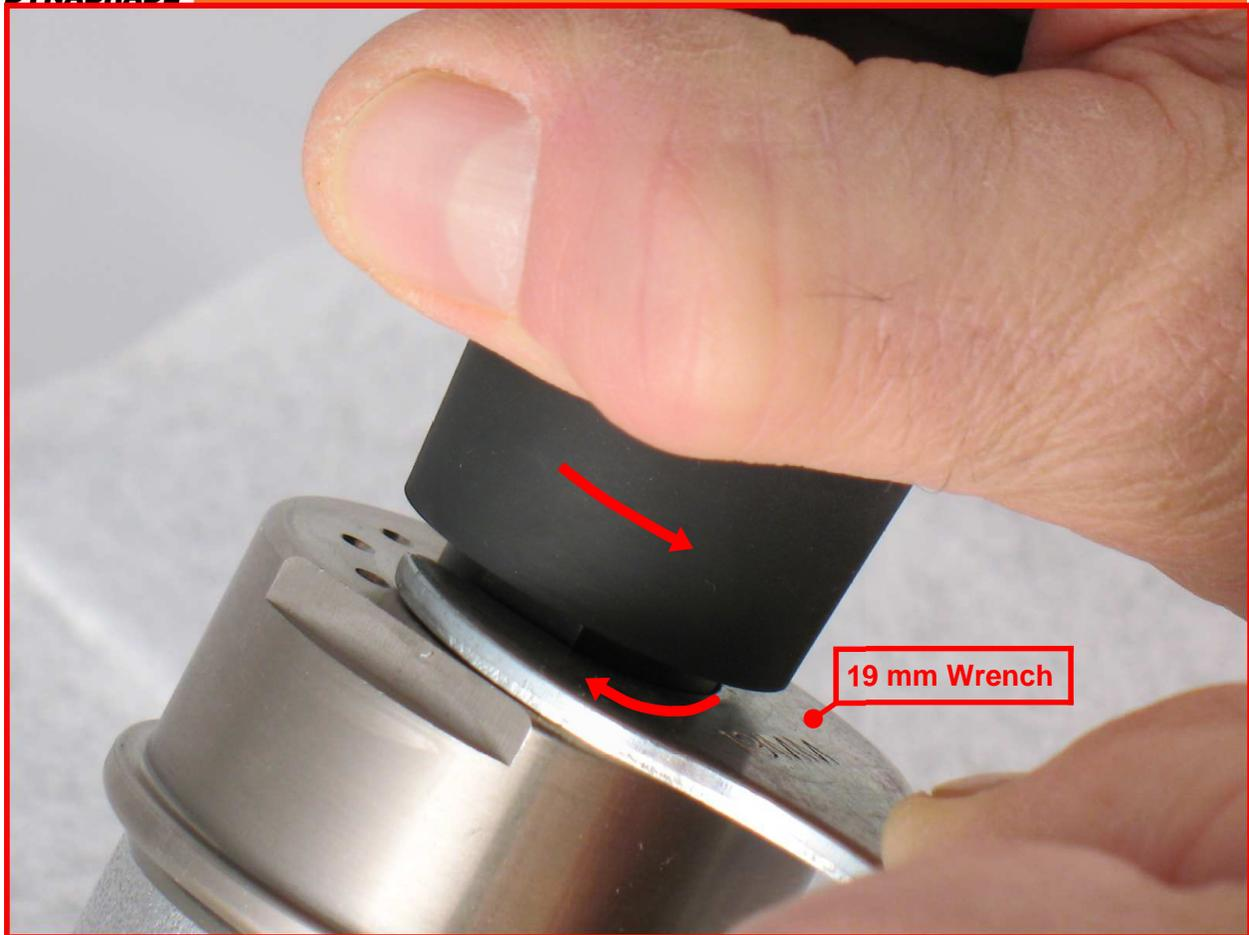
2. Use a 19 mm wrench to hold the motor spindle. By hand, or with groove pliers, grasp the drive wheel and remove it. Turn counterclockwise.
