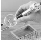
Insert Shaft Lock Tool into spindle hole and open or close the collet with Wrench.
