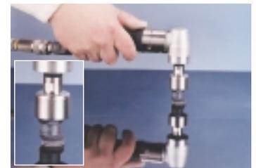
*Excellent for removing dust nibs on clear coat paint systems using various sanding heads and sanding pads.*
