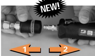
Step One: Pull back on the sleeve and the compressed air is vented. Step Two: Push forward on the sleeve to disconnect the coupler in complete safety!
