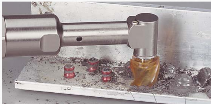
.83" (21 mm) diameter SR Cutter has an internal cavity that fits directly over fasteners for efficient sealant removal.
