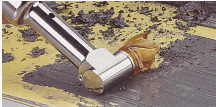
Dynabrade 53455 Right Angle Drill with 3M™ SR Cutter aggressively removes seam sealant.
