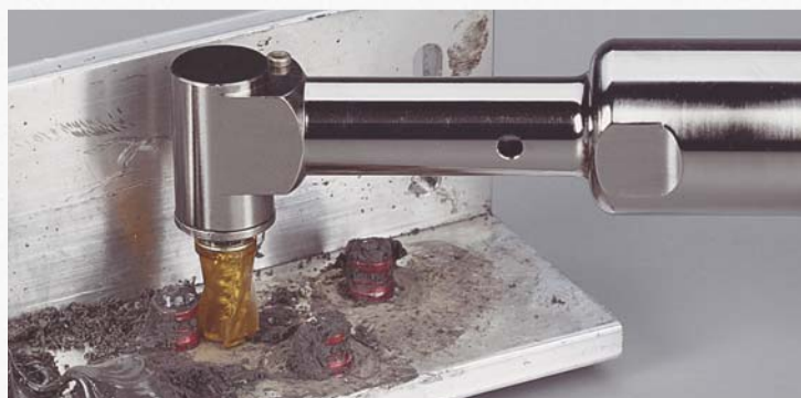
.40" (10 mm) diameter SR Cutter is ideal for working between rivets and in other tight areas.
