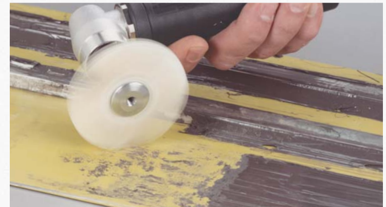
Dynabrade Die Grinder runs 3M™ Radial Bristle Discs for cleaning the final layer of seam sealant. Light pressure is all that is needed!
