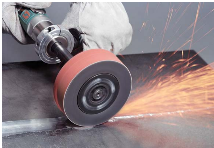
92868 DynaWheel running on 13523 Dynastraight (4,500 RPM) with 13070 Arbor
