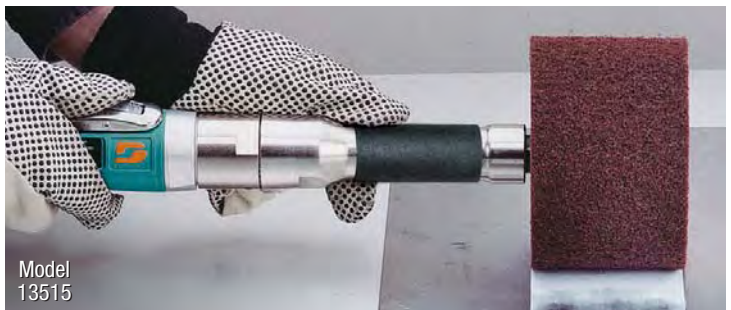
13515 Dynastraight® sets grain pattern in stainless steel.
