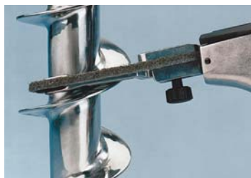
Clean and finish using non-woven nylon belts.
