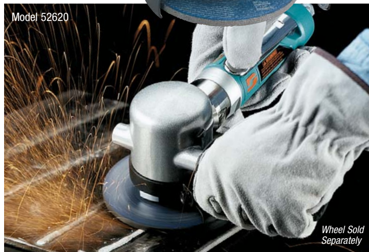
52620 Depressed Center Wheel Grinder takes down a weld.
