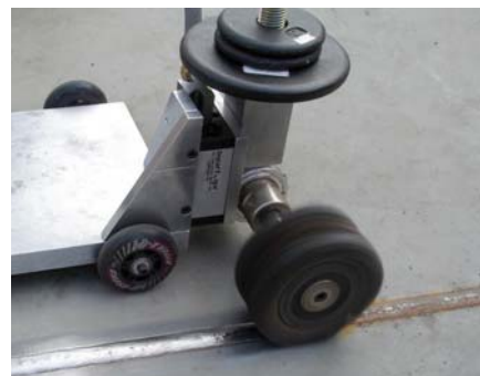
DynaRover cleaning a butt weld. (Shown with optional weight spindle.)
