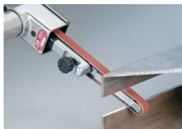
.4 hp Dynafile® II is ideal for deburring and finishing in tight areas.
