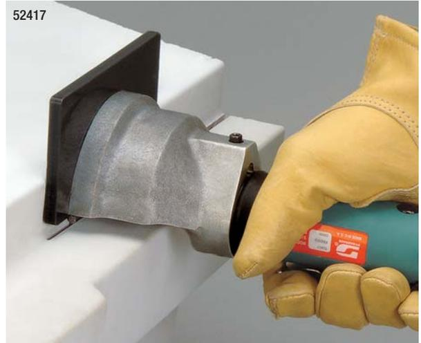
Tool may be operated in horizontal and vertical positions, for flush cutting of edges.
