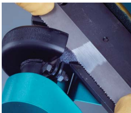
Removing weld slag and excess from gullet (teeth) with cut-off wheel.
