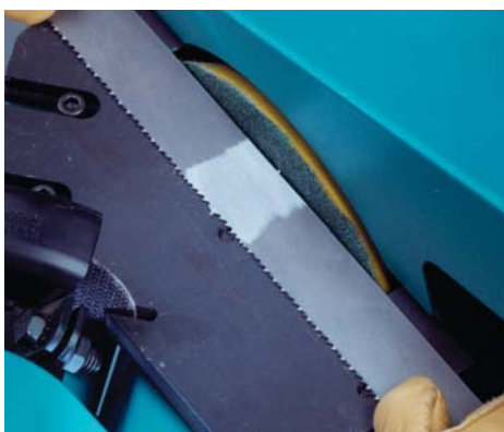
Removing weld slag from back of blade, by contacting it with abrasive disc.
