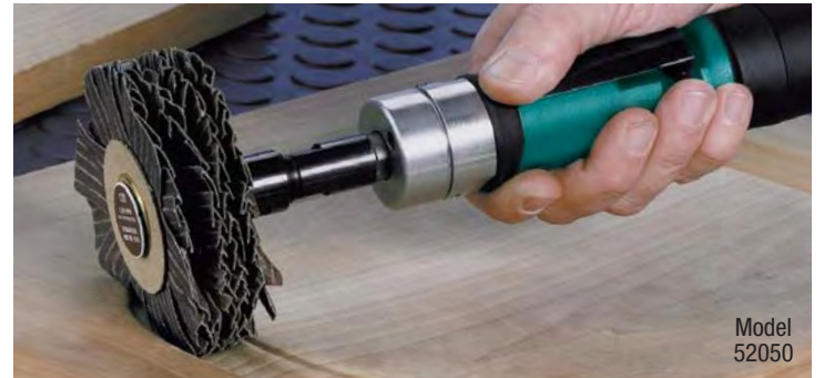
52050 Lightweight Dyninger® with optional spindle-mount stars.
