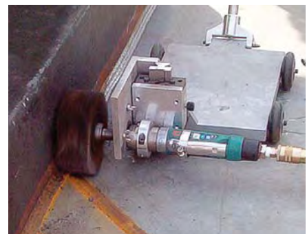
DynaRover cleaning an angle weld.
