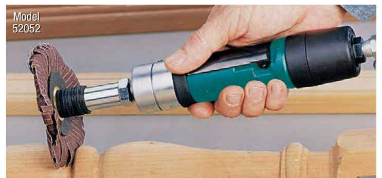
52052 Lightweight Dyninger® with single arbor-mount star attached.
