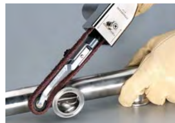
Clean and finish using non-woven nylon belts.
