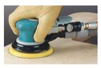
self-generated and central vacuum tools that direct airborne sanding particles away from the operator and the air motor, reducing contamination and the cause of risk to the operator.
