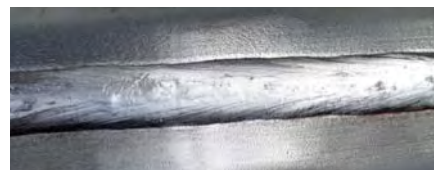
Weld seam cleaned with DynaRover.
