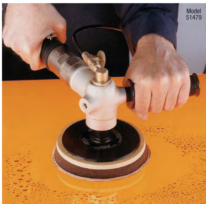
As 51479 is run, water is fed through pad center directly to work surface.
