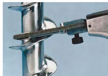
Clean and finish using non-woven nylon belts.
