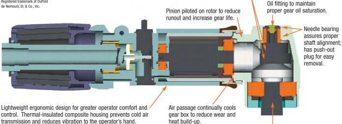
One piece spindle keeps all rotating components on the same centerline to reduce run-out.
