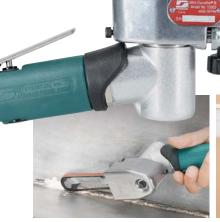
Effective for blending stainless steel and grinding right angle welds.
