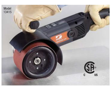
13415 Electric Dynisher® fitted with optional 92938 Dynacushion® Pneumatic Wheel and coated abrasive belt. An ideal setup for achieving in-line scratch pattern on stainless steel.
