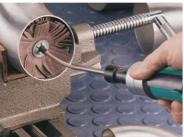
Sand and deburr inside small dia. pipe and other hard to reach areas with 3/4" – 1-1/2" stars. 3" Eyelet Sanding Star easily enters pipe elbow using 7" long flexible mandrel.
