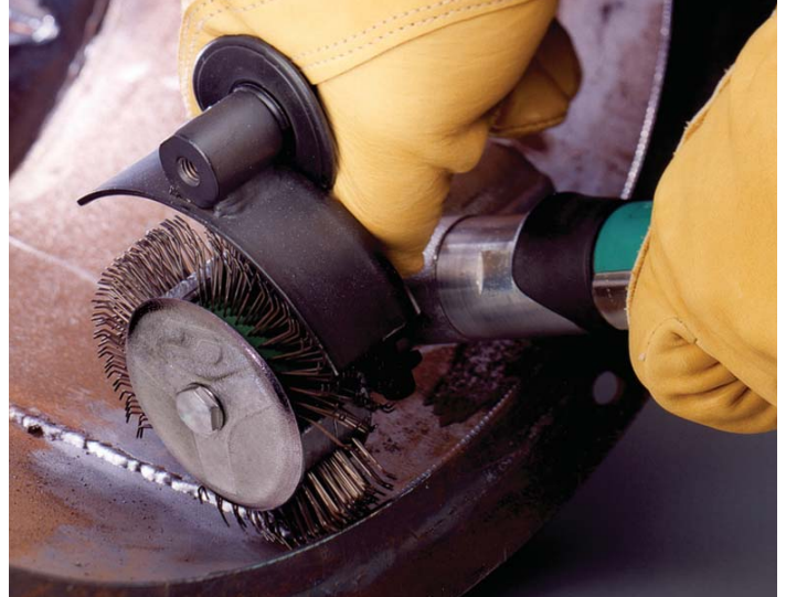
13280 DynaZip powers Wire Wheel to remove surface rust and weld spatter from a weld seam.
