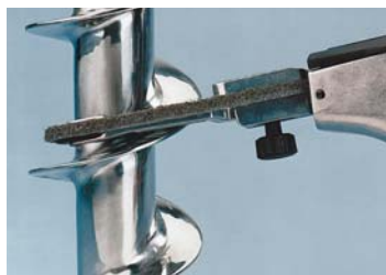
Clean and finish using non-woven nylon belts.
