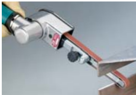
.4 hp Dynaflex® II is ideal for deburring and finishing in tight areas.
