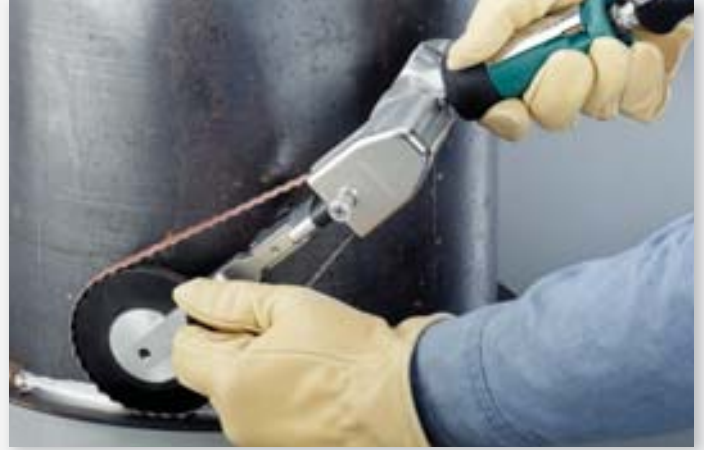
15420 Dynaflex® III includes unique 11702 Contact Arm with 4" (102 mm) diameter wheel, for grinding or blending right angle welds and fillet welds. This arm also comes with helpful hand guide, for enhanced operator control.
