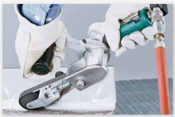
**15300 Dynafile® III** serves up more power for faster material removal. Corner weld shown is easily taken down with optional **15357 Contact Arm**, with "V" shaped Contact Wheel. This arm is also reversible, effective for both platen sanding and slack polishing.
