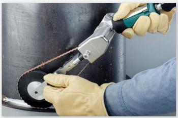
**15420 Dynafile® III** includes unique **11702 Contact Arm** with 4" (102 mm) diameter wheel, for grinding or blending right angle welds and fillet welds. This arm also comes with helpful hand guide, for enhanced operator control.
