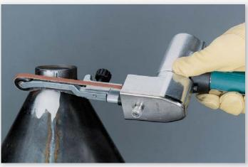
**40320 Dynafile® II** offers ergonomic 7° offset design. The tool's grinding head pivots a full 360° for securing in most efficient position. Application shows **Dynafile® II** fitted with optional **11204 Contact Arm**, allowing slack of abrasive belt to efficiently polish radiused areas.
