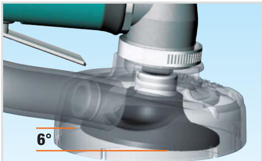
Rendering of 50210 shows 6° angle that ensures ideal contact of abrasive to work surface.
