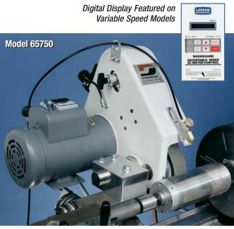
Ideal for use on steel, hard chrome, tungsten carbide, ceramics, thermal spray.
