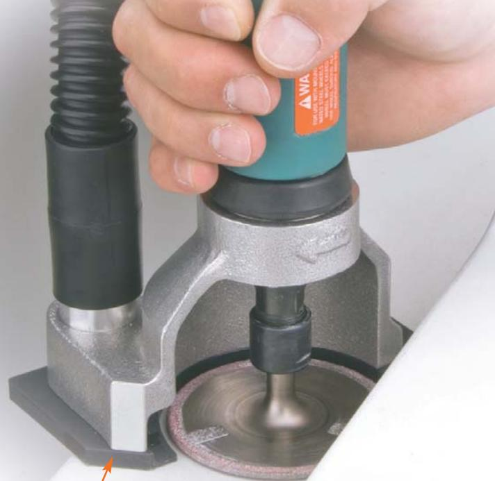
Place this edge against workpiece for consistent cut!
