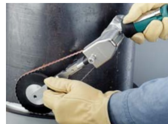
15420 tool (below) includes unique 11702 Contact Arm with hand guide.
