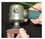
"The spindle won't turn." This usually indicates broken vanes.
