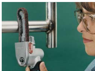
Clean and finish using non-woven nylon belts.
