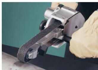
Model 11475 is ideal for grinding circumferential welds.
