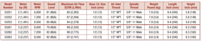
Tune-Up Kit: 2 hp Models - No. 96552; 3 hp Models - No. 96553 (page 267) • Additional Specifications: Air Pressure 90 PSIG (6.2 Bar)
