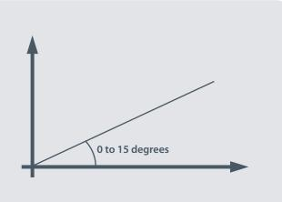
NOTE: Flap discs to be used at an angle of 0 to 15 degrees.
