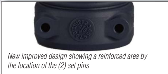
Location of area where failures occurred
