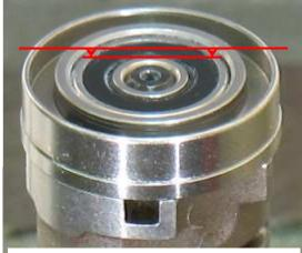
Notice: The rear bearing should sit below the outside surface of the rear bearing plate.
