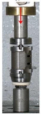
10. Use the RAISED CENTER of the 96242 Bearing Press Tool and the arbor press to install the 02696 Bearing onto the rotor, and into the 02673 Rear Bearing Plate.
